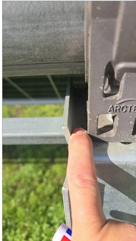
Figure 1 — 11 August 2026. The black plastic bearing, displaced along the torque tube, pushed against the face of the Arctech bearing housing. The finger indicates the contact.
