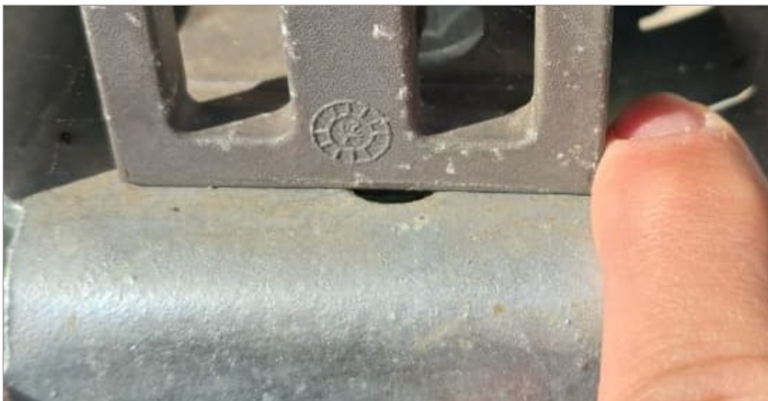
Figure 1 — 11 August 2026. The black plastic bearing, displaced along the torque tube, pushed against the face of the Arctech bearing housing. The finger indicates the contact.
